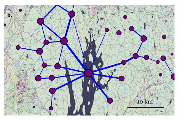
Figure 6. Node importance (purple circles) and link importance (blue lines) at a bandwidth of 10 km, (a) statewide, and (b) focal area. Importance of nodes and links is the loss in regional connectivity that would occur if the node or link were removed. Nodes and links are schematic and do not indicate actual node boundaries nor link paths.
