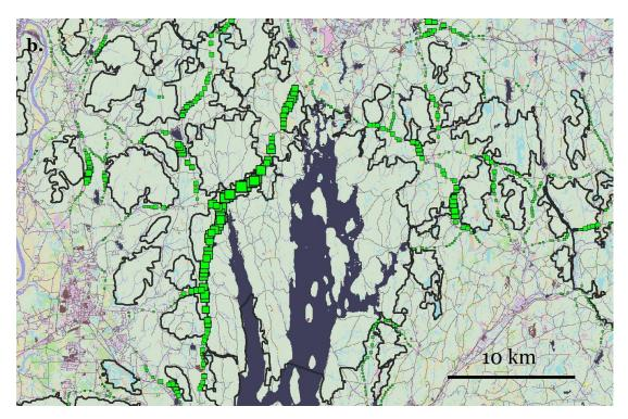
Figure 7. Linkages (green squares) and nodes, (a) statewide, and (b) focal area. The size of the squares indicates the  $\Delta PC$  resulting from installing a road passages structure at each contingent unit. High-valued units indicate places where a road passage structure is expected to make a large contribution to regional connectivity.
