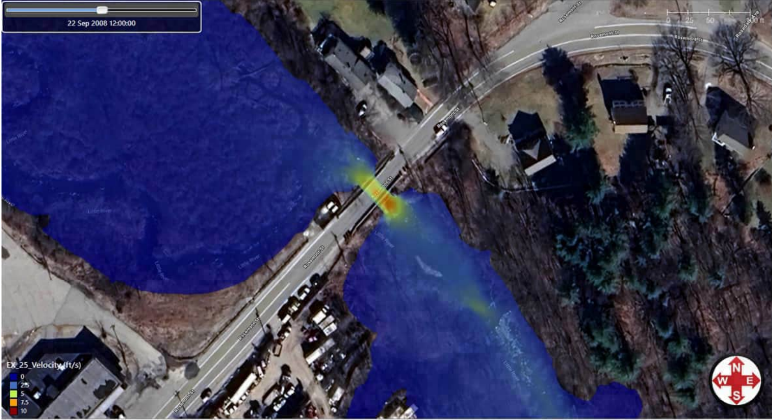
GeoHECRAS 2D Modeling Results: 10-Year Riverine Flood, Existing Conditions.
