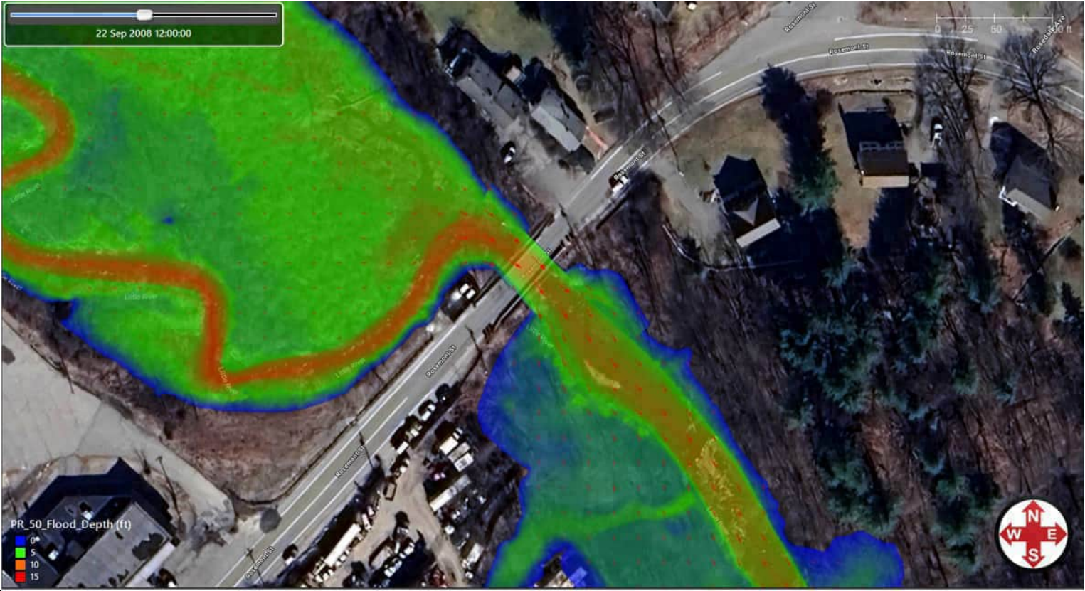
GeoHECRAS 2D Modeling Results: 50-Year Riverine Flood, Proposed Conditions.
