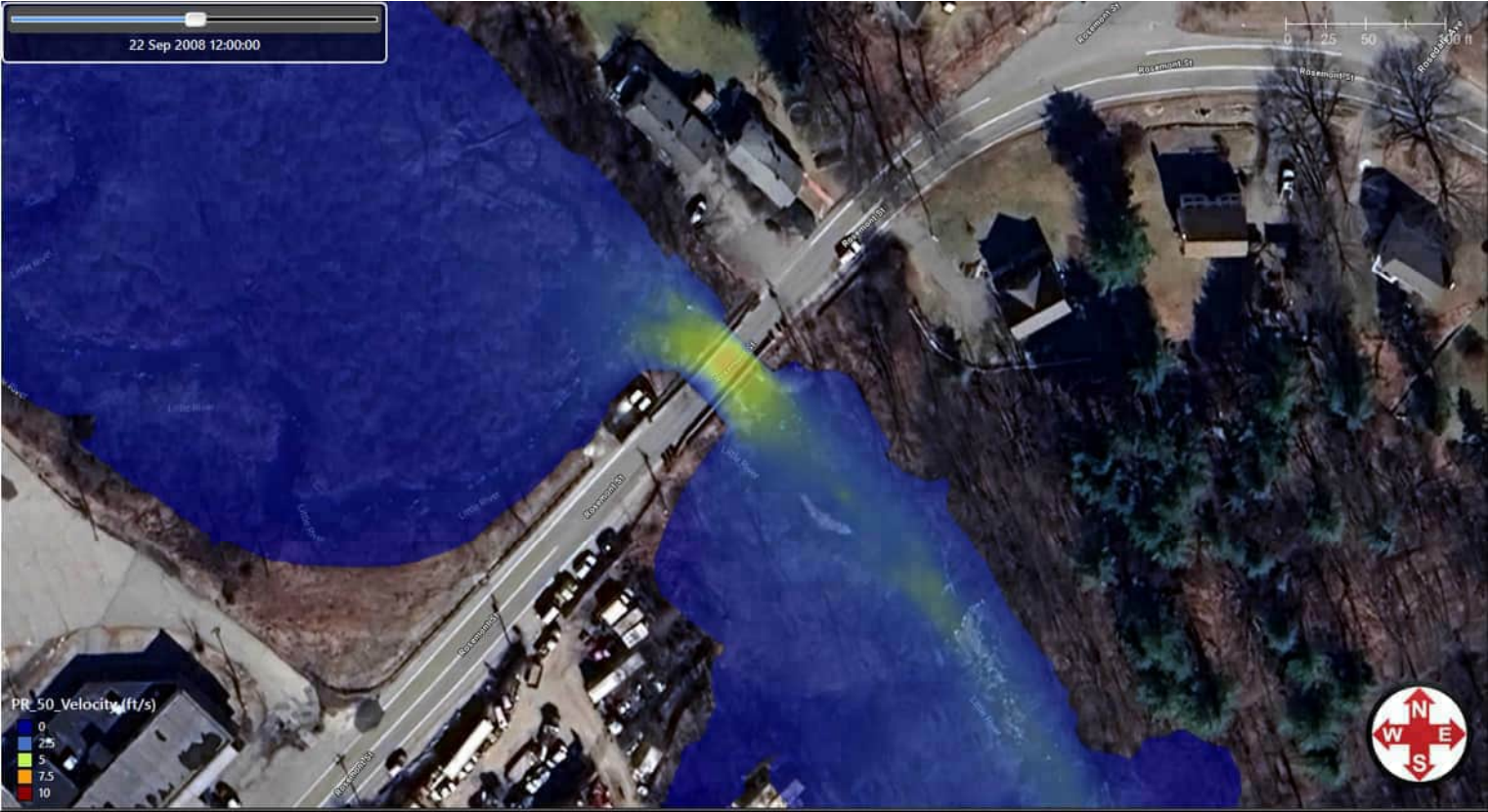
GeoHECRAS 2D Modeling Results: 50-Year Riverine Flood, Proposed Conditions.
