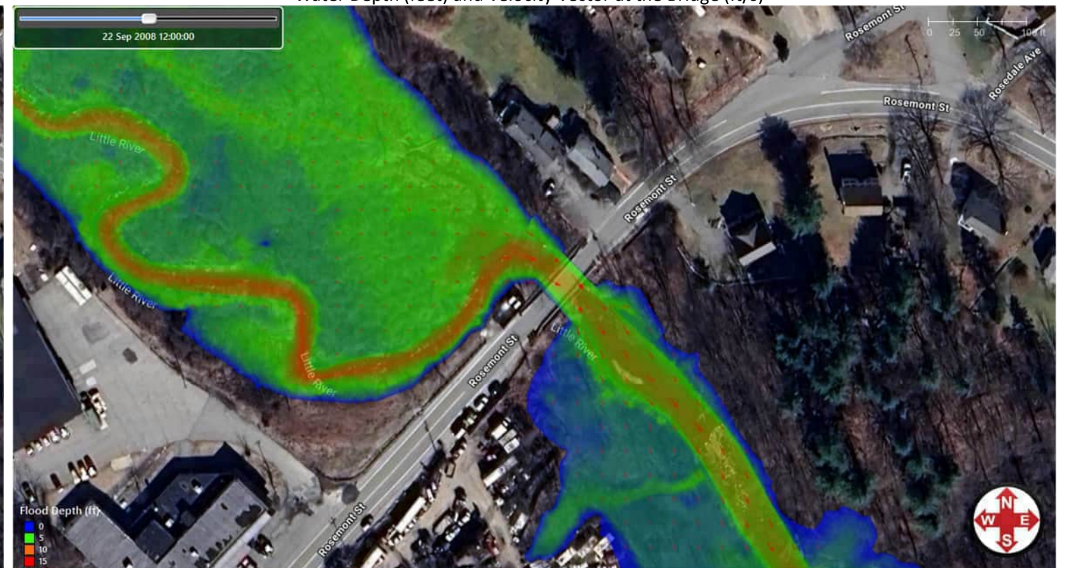
Water Depth (feet) and Velocity Vector at the Bridge (ft/s)
