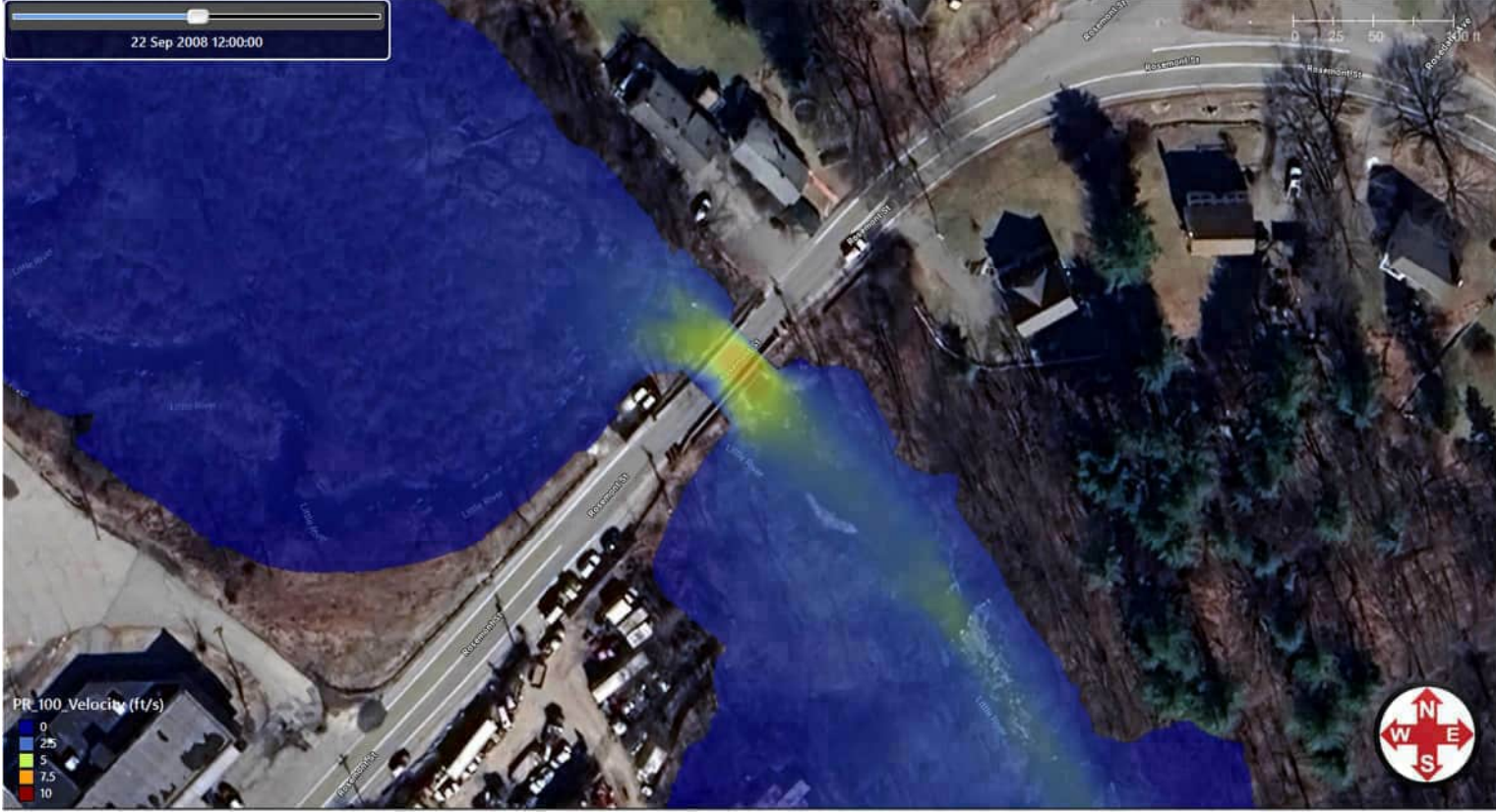
GeoHECRAS 2D Modeling Results: 100-Year Riverine Flood, Proposed Conditions.
