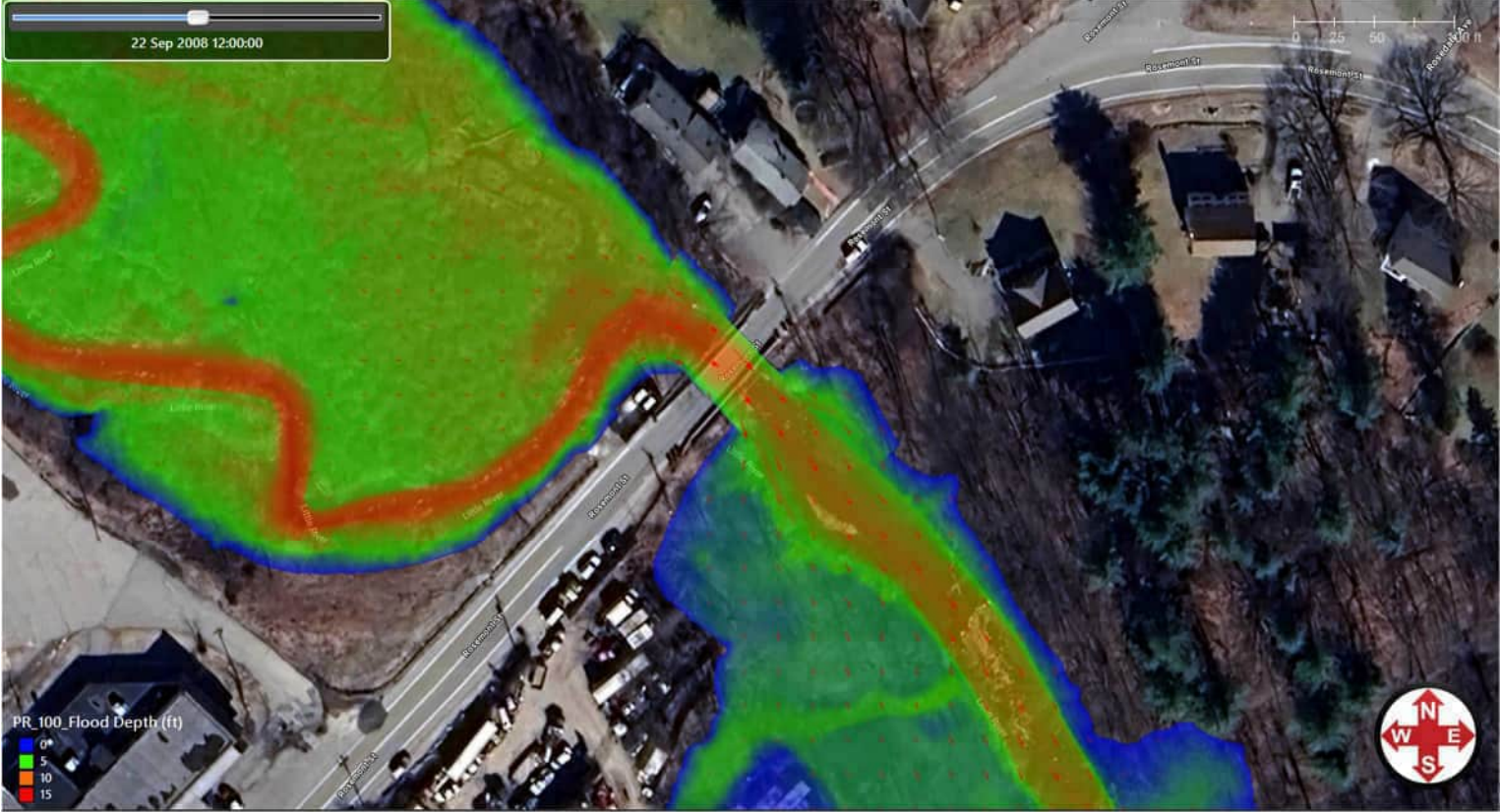
GeoHECRAS 2D Modeling Results: 100-Year Riverine Flood, Proposed Conditions.
