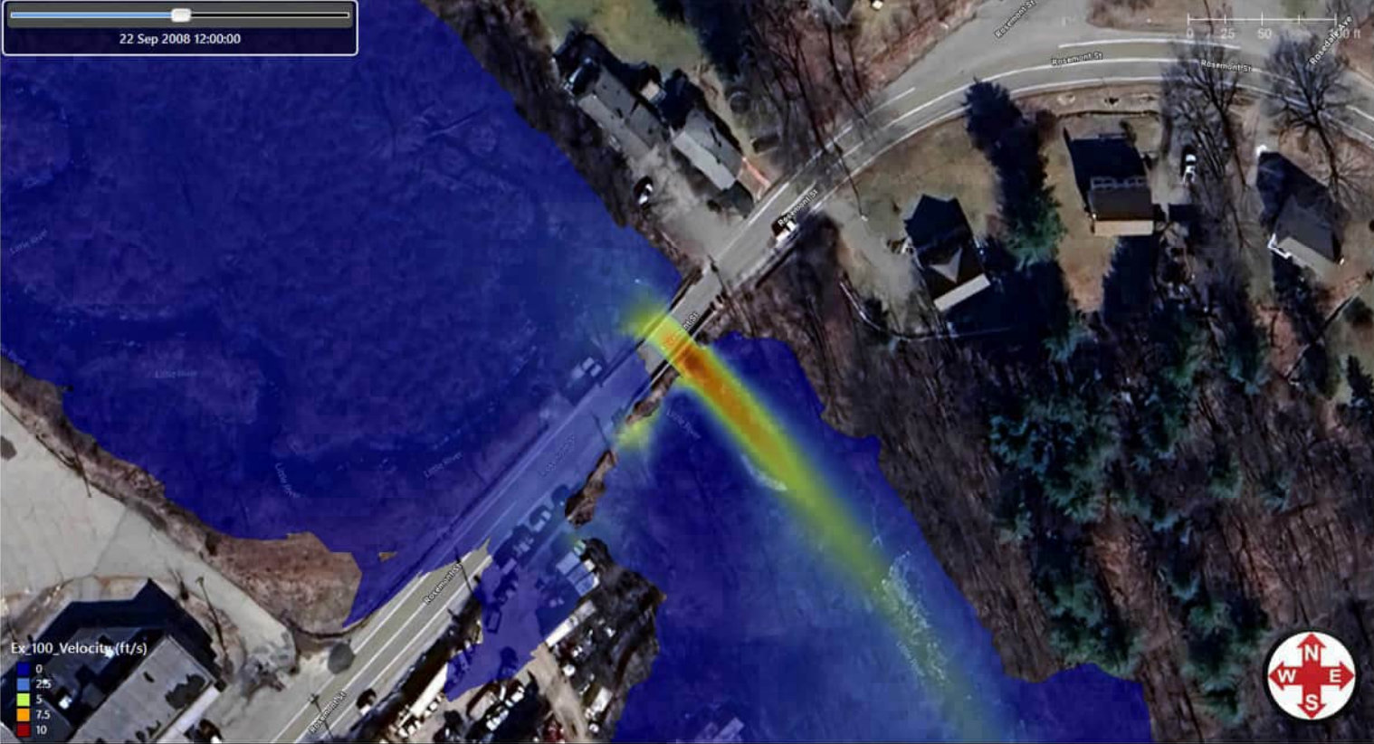
GeoHECRAS 2D Modeling Results: 100-Year Riverine Flood, Existing Conditions.
