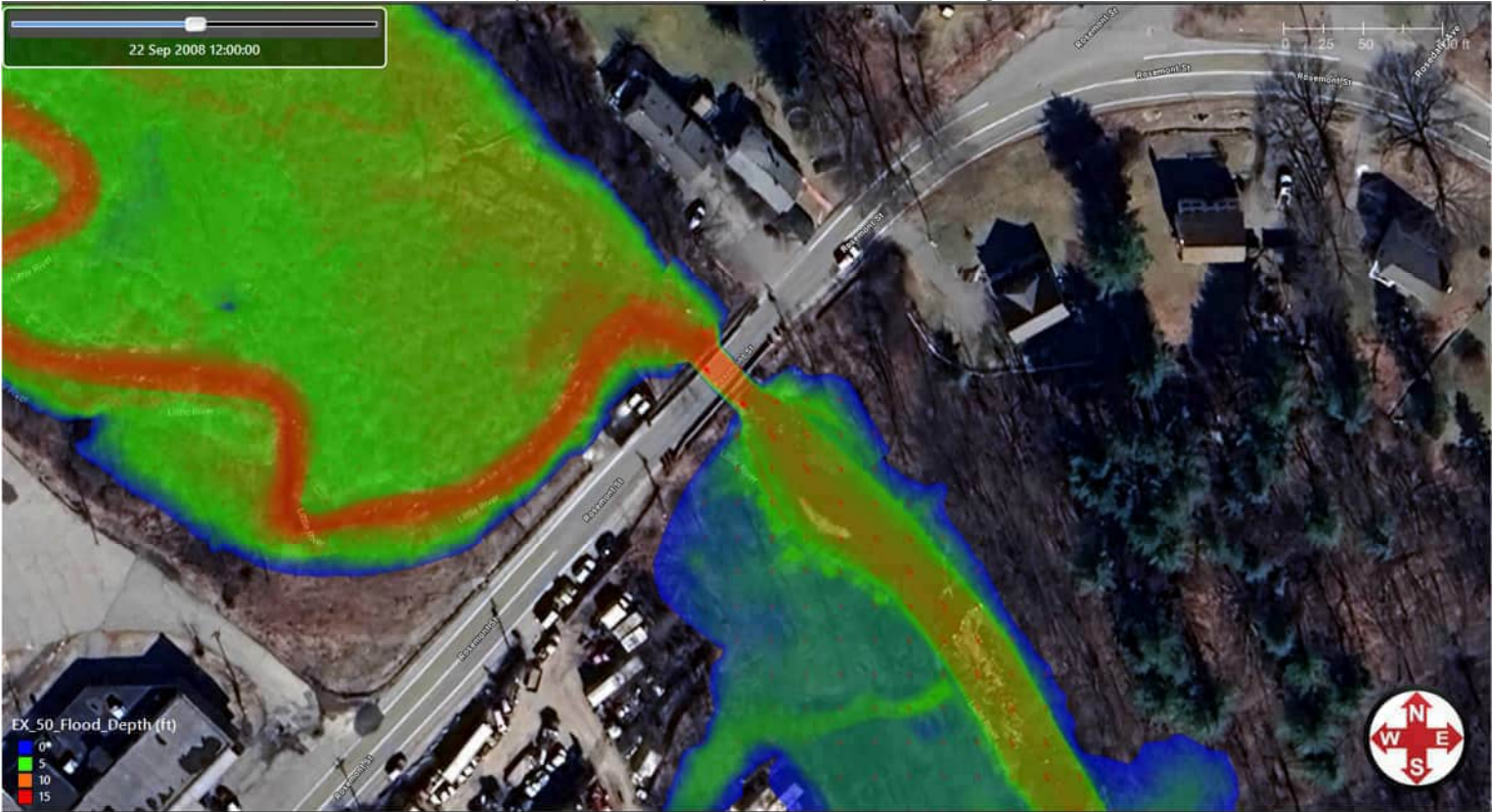
GeoHECRAS 2D Modeling Results: 50-Year Riverine Flood, Existing Conditions.
