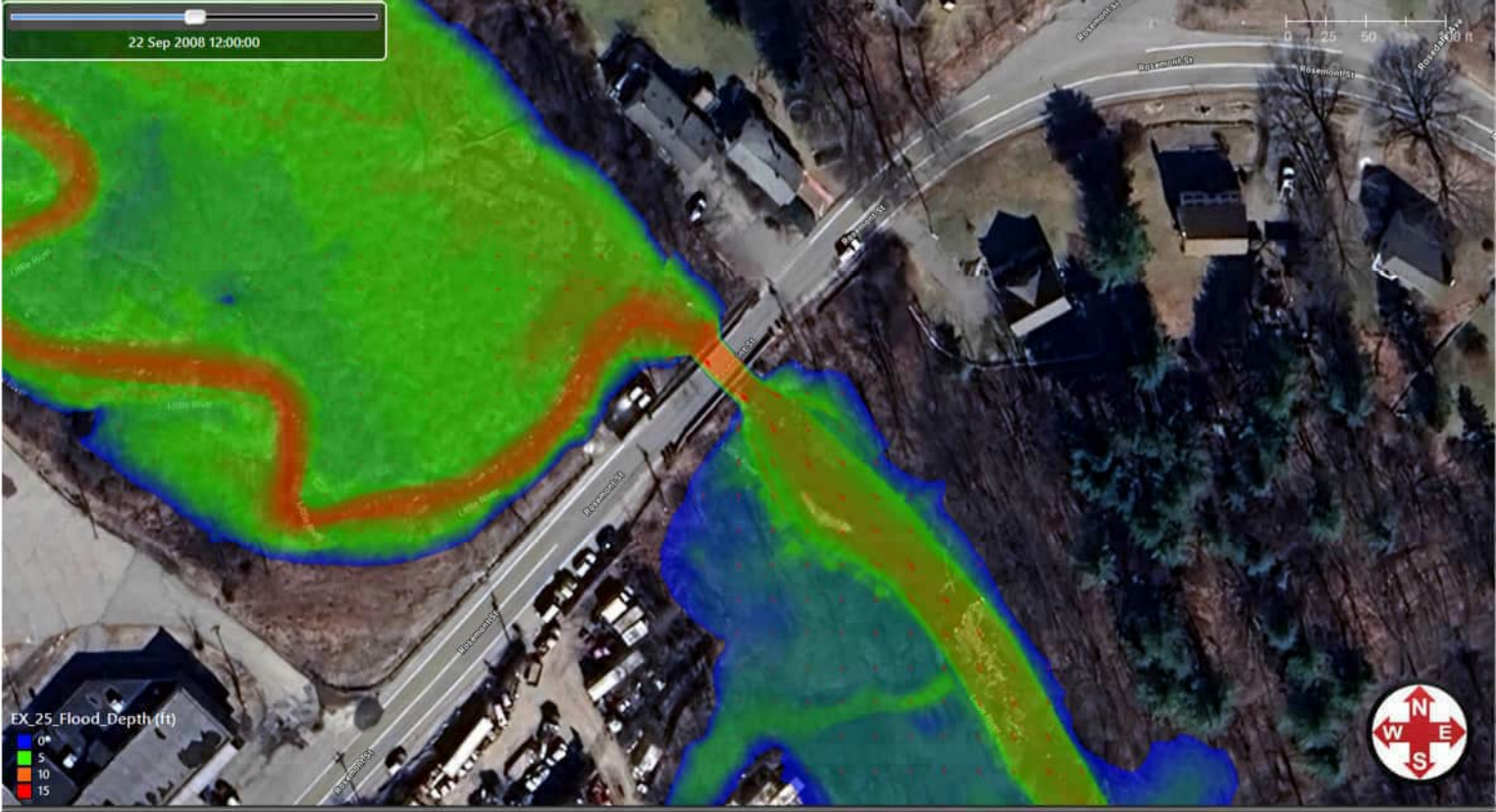
GeoHECRAS 2D Modeling Results: 10-Year Riverine Flood, Existing Conditions.
