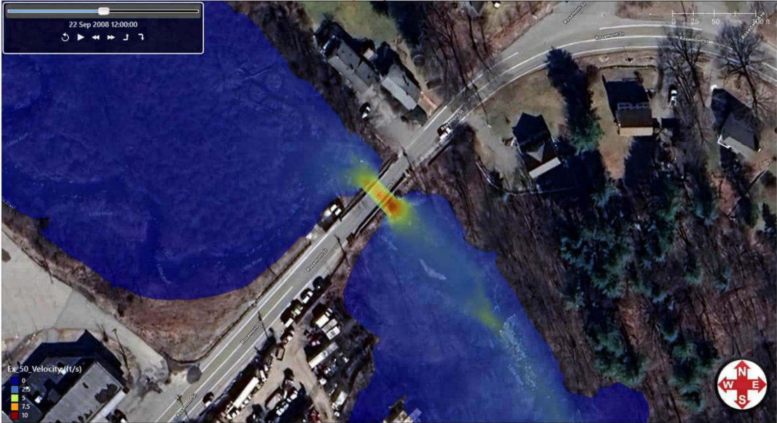
GeoHECRAS 2D Modeling Results: 50-Year Riverine Flood, Existing Conditions.
