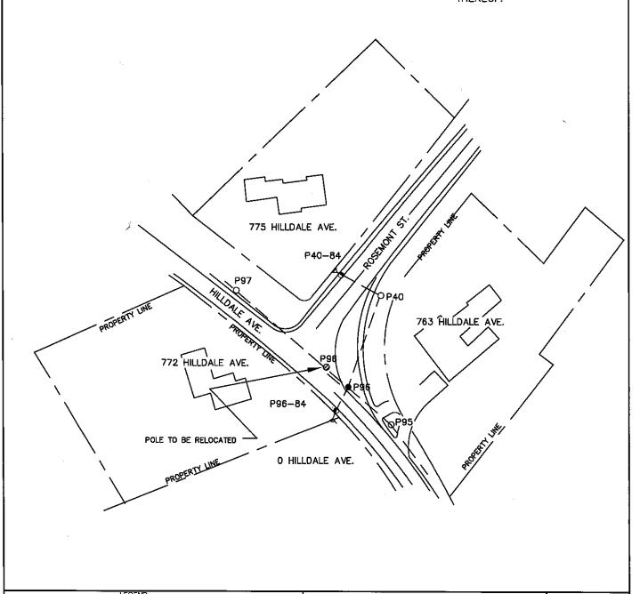
O EXISTING J/O POLE PROPOSED J/O POLE PROPOSED STUB POLE ØJ/O POLE TO BE RELOCATED
