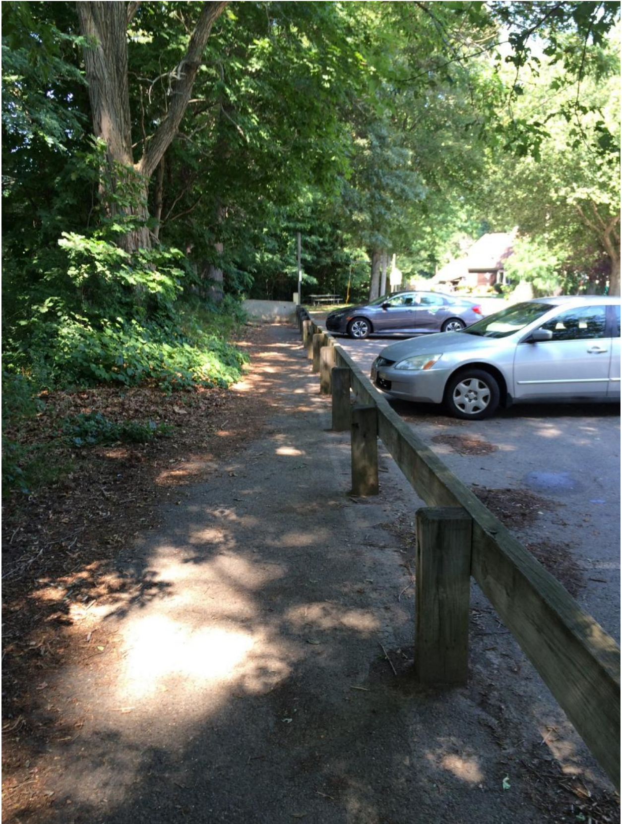
Photo 3: Westerly view of southern parking area where a new walkway will be established within the existing paved parking area footprint. The existing guardrail will be removed and a new wooden guardrail installed north of the walkway. Minor patching of pavement will be required.
